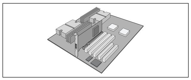
Figure 4-10. QHT7140 Without Riser Installed in a 3U Chassis
